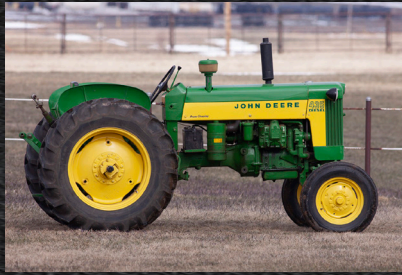
435 John Deere (SN 438476) 2-cylinder Detroit Diesel, 3-point, Single Hydraulic, Power Steering, Showing 1723 hours
