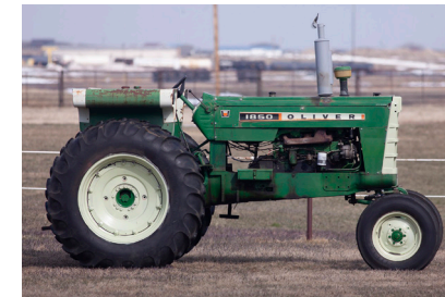
Oliver 1850 (SN 188-769-427) 6-speed Direct Drive, 354 Perkins Diesel Rock Shaft, 2-hydraulics, 3024 hours showing
