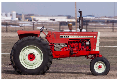
Cockshutt 1650 Diesel (SN 216-912-490) 6-speed Direct Drive, PTO, 2-hydraulics, 6862 hours, 3-speed Hydraul and 3-point arms, will go with the tractor all on a pallet, has Rockshaft
