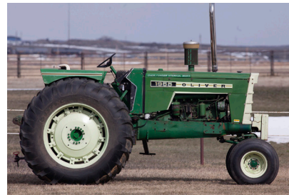
Oliver 1955 (SN 251-557-692) 3-speed Hydraul, 2-PTO's, 2-hydraulics, 3-point, 4398 hours
