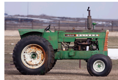
Oliver 1850 Wheatland (SN 175-220-427) 2-speed Hydra Power, PTO, 2-hydraulics, 354 Perkins Diesel, Runs & Drives, Engine has 1 cylinder not firing properly
