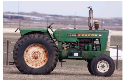
Oliver 1900 Wheatland Diesel (SN 134-356-950) 2-speed Hydra Power, 2-hydraulics, 4-cylinder Detroit, 6836 hours
