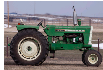
Oliver 1850 Diesel (SN 200-877-528) 3-speed Hydraul, 3-point, 2-hydraulics, Dual PTO's, 3185 hrs.
